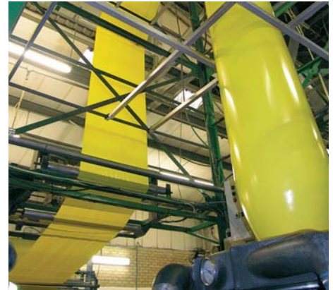
Blown extrusion line
